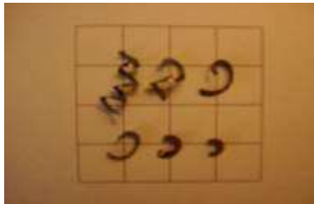
C-type and \epsilon -type broken chips
