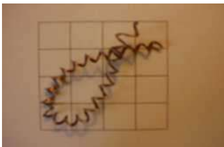
Long helical unbroken chips
