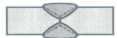
Double V-groove weld for thicker sections
