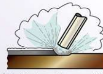
Shielded metal arc welding
