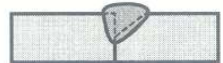
Single bevel groove weld
