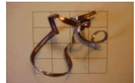
Long and snarled unbroken chips
