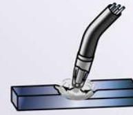
Gas-metal arc welding
