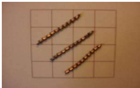
Medium helical broken chips
