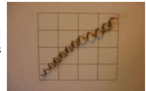
Long helical broken chips
